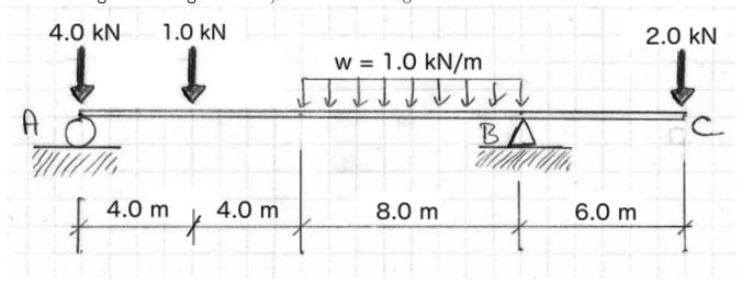
(a) Find the support forces  $A_y$ ,  $B_x$ , and  $B_y$  exerted on the beam by supports A and B.
