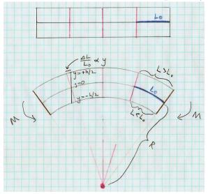
Next, use the symbol e to denote the axial strain  $\Delta L/L_0$ , and use the symbol f to denote stress, which is force/area. For an elastic material, f = eE, where E is Young's modulus. So we have  $y/R = \Delta L/L_0 = e = f/E$ . So the axial stress (force per unit area) exerted by the fibers a distance y above the neutral axis is f = Ey/R.
