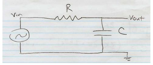
**Problem 3.** Look again at the low-pass filter from problem 2, with R=2.5K and C=.068 $\mu$ F. What happens to |Vout/Vin| if you place a 250K load resistor in parallel with C? Now what happens if you place a 2.5K load resistor in parallel with C? What is |Vout/Vin| at DC now? What is  $f_{3dB}$  now?
