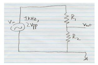
**Problem 2.** Look again at the circuit from problem 1(d). Does it make any difference that f=1kHz? Now replace R2 with a .068µF capacitor. Calculate |Vout/Vin| for f=0Hz (i.e. for DC), f=100Hz, f=1kHz, f=10kHz, f=1MHz. (Remember that  $f=\omega/2\pi$ .) At what limit (in frequency) is |Vout/Vin| maximized? What is this maximum value? At what frequency does |Vout/Vin| fall to  $1/\sqrt{2} \approx 0.707$  of its maximum?
