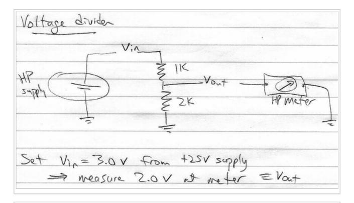
Vth = voltope with Read = po. Since Rin of meter = 10 MR >> RH (as we will see balow), the meter is directly measuring Vth. VHL = 2.0V. By calculation, VHL = Vin Rithe =3V2K = 2V. OK. Ryh = current with Real=0. Since Rishunt of ammeter = 52 (from pant I) << RH (we'll show meter is effectively a short circuit. Put meter in DC current mode -> measure 3.0 mA. Rth = Vth/Isc = 2V/3mA = 670.2. Calculate: Rth = 1K 2K = (2K (2K) 2K= Load dividen of 100K resistor:
