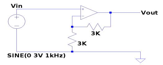
Now insert your non-inverting amplifier where the inverting amp was before (and where the follower was before that). What are Vb1 and Vb2 in this configuration? What do you infer about the input impedance of the non-inverting amplifier circuit?
