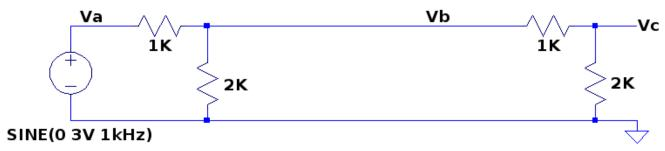
Recall that the second divider loads the first divider, reducing Vb from 2V to about 1.64V in amplitude. Now insert the follower between the first divider and the second:
