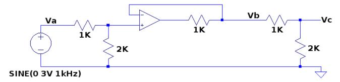
Now how large is Vb? What do you infer about the follwer's output impedance now? In effect, you have shown that even if you changed the output impedance of the opamp itself to 1K, the feedback would cause the output impedance of the follower as a whole to be far less than 1K. The power of feedback! Are you impressed?
