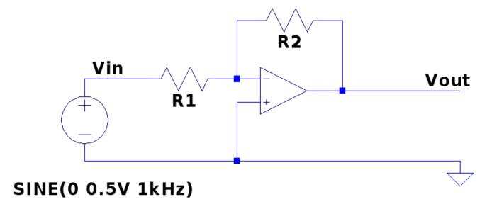
Now choose resistors for a gain of -10. Try 1Vpp inputs; look at Vout. Now try 5Vpp inputs. What happens? Now go back to 1Vpp sine waves and try increasing the frequency. Notice that the ideal behavior breaks down once you get up beyond a few hundred kHz – see data sheet if you're curious. (We'll discuss opamp real life next week.)
