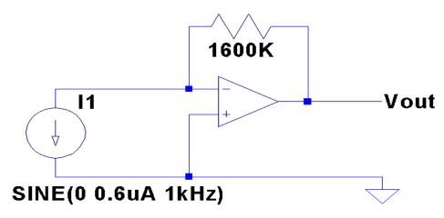
The idea, if all goes well, is for you to drive an LED (protected by a resistor) with the function generator, and then to detect that light with the photodiode, whose signal you will amplify and display on the scope. A rough illustration is shown below – though the details remain to be worked out.
