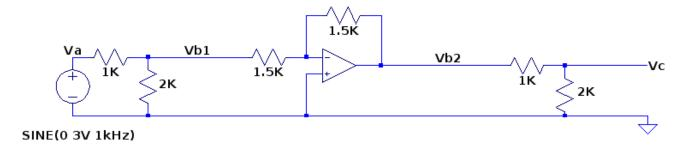
Now replace the two 1.5K resistors with 33K resistors. What happens to Vb1 and Vb2? Do you see how the input impedance of the inverting configuration depends on the resistor choices?
