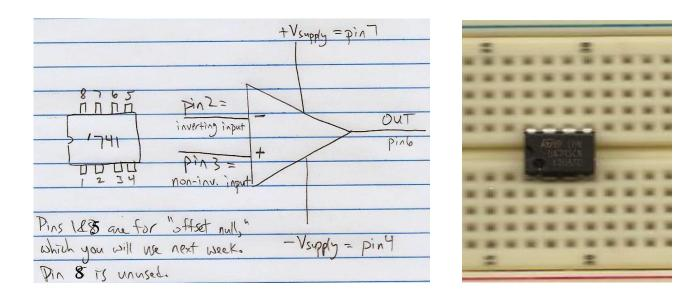
First get to know the conventional 8-pin opamp DIP pinout, illustrated above. Connect a '741 on your breadboard as shown, so that the breadboard does not short any of the opamp's pins together.
