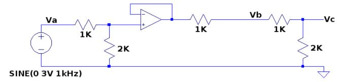
How does 1K compare with the input impedance of the second divider? How large is Vb now? (You should calculate in your head the answer you expect before you measure it!) Clearly a 1K output impedance makes it difficult to drive the 3K input impedance of the second divider without sagging.
