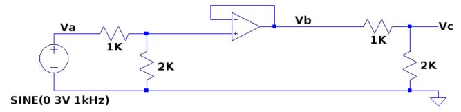
Voilà! No more loading. You should see 2V amplitude at Vb now, which is what you saw in Lab 1 when the second divider's resistors were chosen to be large enough (100K:200K) to produce negligible loading.
