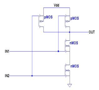
inverter. So NOT (A NAND B) gives you (A AND B). And ((NOT A) NAND (NOT B)) gives you A NOR B. And NOT (A NOR B) then gives you (A OR B). So with a NAND gate, you can do it all.
