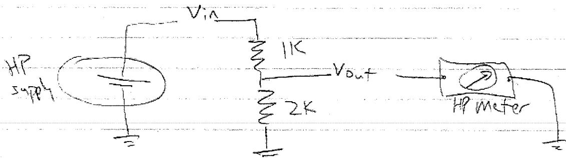
Set  $V_{in} = 3.0\text{ V}$  from +25V supply
