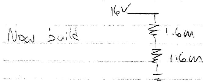
I inserted ammeter between lower resistor & ground. Measure  $\approx 5 \mu\text{A}$ .
