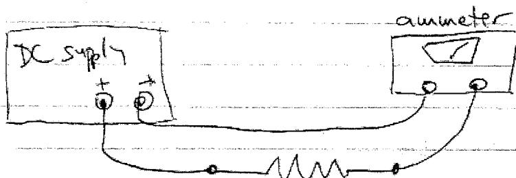
Setup for measuring  $I$  vs.  $V$
