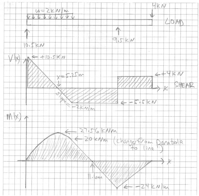
(c) What are the largest magnitude of the shear V (in kilonewtons) and the largest magnitude of the bending moment M (in kilonewton-meters)?
