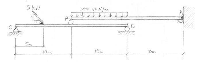
(a) Draw an extended free-body diagram for the upper beam, indicating all forces acting on the beam, their directions, and their lines of action. In this diagram, replace the distributed load with an equivalent point load. (It's "equivalent" for the purpose of finding the support forces.)
