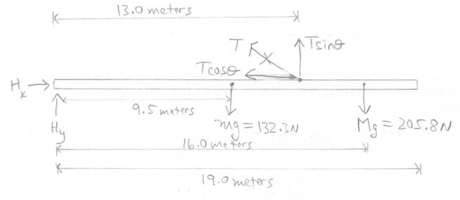
(b) Find the tension T in the diagonal guy wire and the forces  $F_x$  and  $F_y$  exerted by the hinge on the beam. (Remember that forces are in newtons, while masses are in kilograms.)
