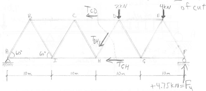
(a) Find the force  $F_{y}$  exerted on the truss by the roller support at F.
