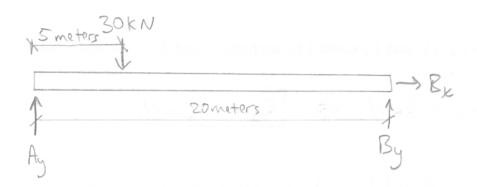
(b) Find the support forces  $A_y$ ,  $B_x$ , and  $B_y$  exerted by supports A and B on the upper beam.
