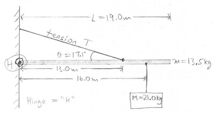
(a) Draw an extended free-body diagram for the beam, indicating all forces acting on the beam, their directions, and their lines of action. Don't forget the mass of the beam itself.
