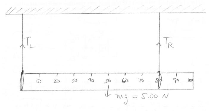
(a) What is the tension in the string at 80 cm? (I mean the tension in the straight part of the string that is above the ruler; don't worry about the small portion that encircles the ruler.)
