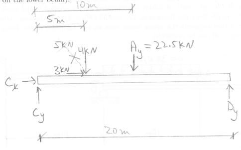
(d) Find the support forces  $C_x$ ,  $C_y$ , and  $D_y$  exerted by supports C and D on the lower beam.
