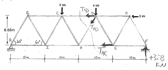
(a) Find the force  $F_y$  exerted on the truss by the roller support at F.
