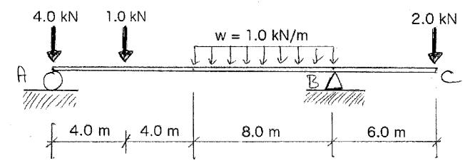
(a) Find the support forces  $A_y$ ,  $B_x$ , and  $B_y$  exerted on the beam by supports A and B.
