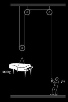
A piano mover raises a 100 kg piano at a constant speed using the pulley system shown here. With how much force is she pulling on the rope? (Ignore friction and assume  $g \approx 10 \text{ m/s}^2$ .) (A) 2000 N (B) 1500 N (C) 1000 N (D) 750 N (E) 500 N (F) 200 N (G) 50 N (H) impossible to determine.
