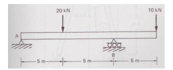
**4\*.** Find the "reaction" forces exerted by the supports **A** and **B** on the beam in the right figure above. (There are three forces to find: two vertical and one horizontal.)
