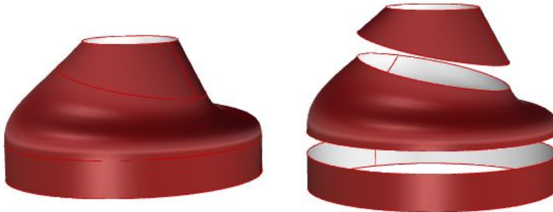
Figure (70): Polysurfaces are made out of joined surfaces with common edges aligning perfectly within tolerance.
