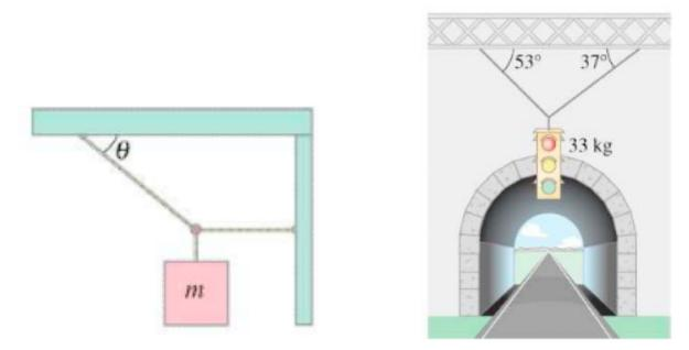
9. Find the tension in the two wires supporting the traffic light shown in the figure above (right).
