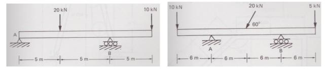
11<sup>\*</sup>. Find the "reaction" forces exerted by the supports A and B on the beam in the right figure above. (There are three forces to find: two vertical and one horizontal.)
