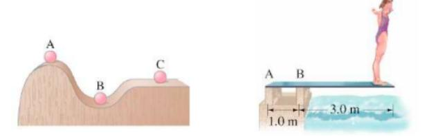
7. Calculate the forces (magnitudes and directions)  $F_A$  and  $F_B$  that the supports exert on the diving board in the figure above (right) when a 59 kg person stands at its tip. (a) Ignore the weight of the board. (b) Take into account the board's mass of 23 kg. Assume the board's CoM is at its center.
