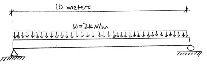
(a) Find the support forces  $L_x$ ,  $L_y$ , and  $R_y$  exerted on the beam by the left ("L") and right ("R") supports.
