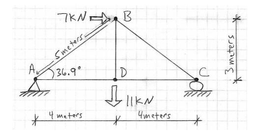
(a) Using static equilibrium of the truss as a whole, solve for the support forces  $A_x$  and  $A_y$  exerted on the truss by the hinge support at A and for the support force  $C_y$  exerted on the truss by the roller support at C. Be sure to indicate whether  $A_x$  points left or right and whether  $A_y$  and  $C_y$  point up or down.
