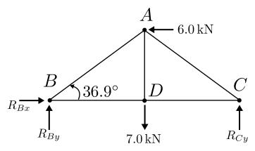
(d) Using the method of joints, write  $\sum F_y$  for joint C to solve for the bar tension  $T_{AC}$ . Indicate whether bar AC is in tension or in compression. As a check against careless mistakes, you should expect your answer to be one of the following:  $\pm 1.250 \text{ kN}$ ,  $\pm 1.667 \text{ kN}$ ,  $\pm 2.083 \text{ kN}$ ,  $\pm 5.750 \text{ kN}$ ,  $\pm 6.000 \text{ kN}$ ,  $\pm 7.000 \text{ kN}$ ,  $\pm 9.583 \text{ kN}$ .
