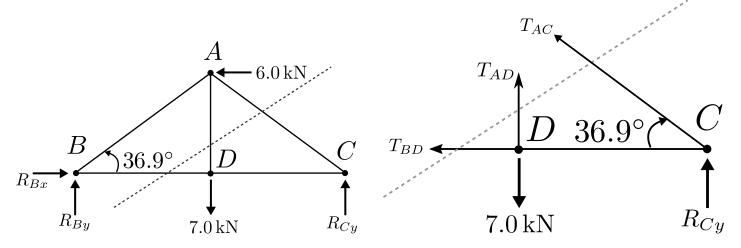
(j) Using moments about joint D, write an equation that lets you check the consistency of your results for  $T_{AC}$  and  $R_{Cy}$ . (Alas, this equation may feel a bit redunant to you.)
