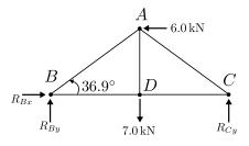
(g) Using the method of joints, write  $\sum F_x$  for joint C to solve for the bar tension  $|T_{CD}|$ . Indicate whether bar CD is in tension or in compression. As a check against careless mistakes, you should expect your answer to be one of the following:  $\pm 1.250 \text{ kN}$ ,  $\pm 1.667 \text{ kN}$ ,  $\pm 2.083 \text{ kN}$ ,  $\pm 5.750 \text{ kN}$ ,  $\pm 6.000 \text{ kN}$ ,  $\pm 7.000 \text{ kN}$ ,  $\pm 9.583 \text{ kN}$ .
