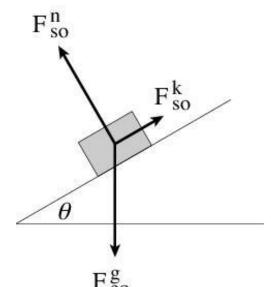
An object "O" of mass m slides down an inclined surface "S" at constant velocity. Let the x-axis point downhill. What is the magnitude of the **downhill (tangential) component**  $F_{eo,x}^g$  of the gravitational force exerted by Earth on the object?
