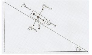
Magnitude of "normal" force ("normal" is a synonym for "perpendicular") between surfaces is
