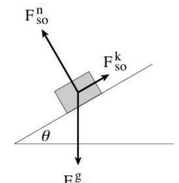
Since object "O" slides down surface "S" at constant velocity, the forces on O must sum vectorially to zero. How do I express this fact for the forces acting along the downhill (tangential) axis?
