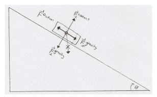
Block begins sliding when downhill component of gravity equals maximum magnitude of static friction:
