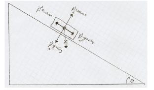
Take x-axis to be downhill, y-axis to be upward  $\perp$  from surface.
