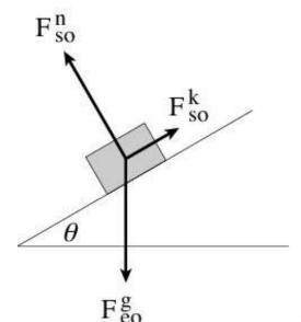
An object "O" of mass m slides down an inclined surface "S" at constant velocity. What is the magnitude of the (kinetic) **frictional force**  $F_{so}^k$  exerted by the surface on the object?
