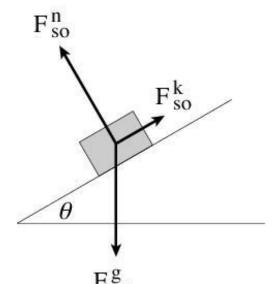
An object "O" of mass m slides down an inclined surface "S" at constant velocity. What is the magnitude of the **gravitational** force  $F_{eo}^g$  exerted by Earth on the object?
