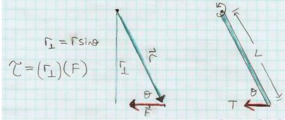
Alternative method: use  $(r)(F_{\perp})$  instead of  $(r_{\perp})(F)$ .
