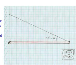
A beam of mass  $M=20~\mathrm{kg}$  and length  $L=2~\mathrm{m}$  is attached to a wall by a hinge. A sign of mass  $m=10~\mathrm{kg}$  hangs from the end of the beam. The end of the beam is supported by a cable (at  $\theta=30^\circ$  angle w.r.t. horizontal beam), which is anchored to the wall above the hinge.
