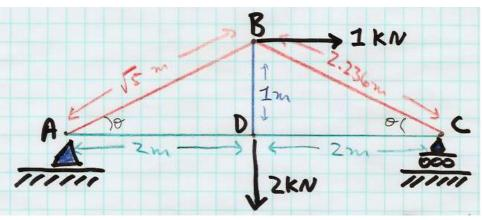
How many equations does the "method of joints" allow us to write down for this truss? (Consider how many joints the truss has.)
