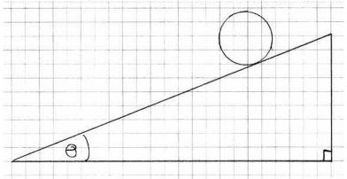
What 3 forces act on the cylinder? What is the rotation axis? Draw FBD and extended FBD. What are the torque(s) about this axis? How are  $\alpha$  and a related? Write  $\vec{F} = m\vec{a}$  and  $\tau = I\alpha$ .
