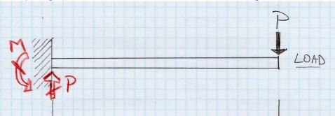
Sign conventions: V>0 when beam LHS section is pulling up on beam RHS; M>0 when beam is smiling.
