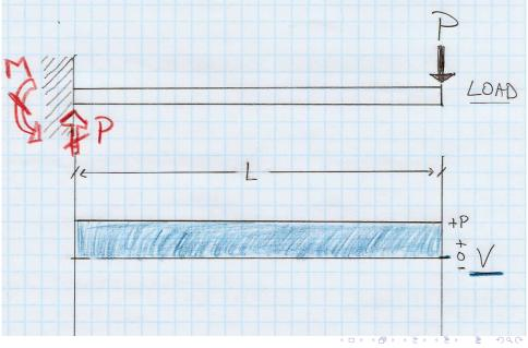
Sign conventions: V>0 when beam LHS section is pulling up on beam RHS; M>0 when beam is smiling.
