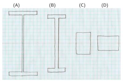
Each shape has same area  $A=24~\rm cm^2$ , but "second moment of area" is  $I_A=1328~\rm cm^4$ ,  $I_B=792~\rm cm^4$ ,  $I_C=72~\rm cm^4$ ,  $I_D=32~\rm cm^4$ . That's the motivation for the "I" shape of an I-beam: to get a large "second moment of area,"  $I=\int y^2 \, \mathrm{d}A$ . The deflection of a beam under load is inversely proportional to I.
