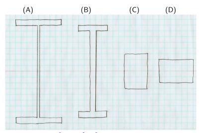
Given that  $I_x = \int y^2 dA = \frac{1}{12}bh^3$  for a rectangle centered at y = 0, let's use the parallel-axis theorem to calculate  $I_x$  for shapes A, B, C, and D. For definiteness, let each graph-paper box be  $1 \text{ cm} \times 1 \text{ cm}$ . So the units will be  $\text{cm}^4$ .
