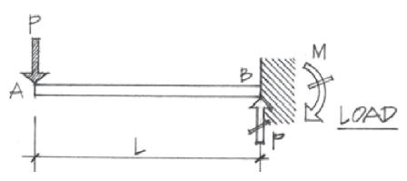
Sign conventions: V > 0 when beam LHS section is pulling up on beam RHS; M > 0 when beam is smiling.
