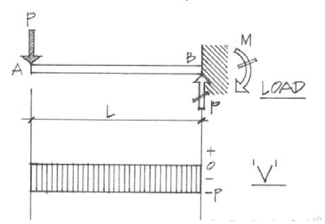
Sign conventions: V>0 when beam LHS section is pulling up on beam RHS; M>0 when beam is smiling.
