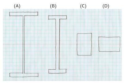
Each shape has the same area: 24 squares. Which shape has the largest  $I_x = \int y^2 dA$  ("second moment of area about the x-axis"), with y = 0 given by the faint horizontal red line at the center?
