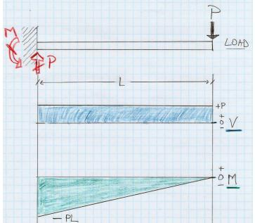
Let's try a mirror image of the same cantilever beam. Sign conventions: V>0 when beam LHS section is pulling up on beam RHS; M>0 when beam is smiling.
