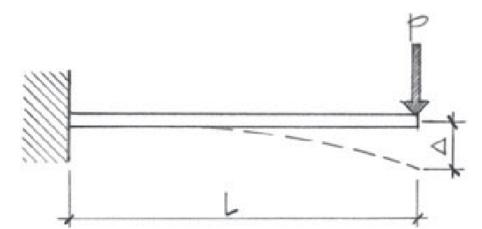
We draw "load diagram" (basically a FBD for the beam), then the "shear (V) diagram" below that, then the "moment (M) diagram" below that. Sign conventions: V>0 when beam LHS section is pulling up on beam RHS; M>0 when beam is smiling.
