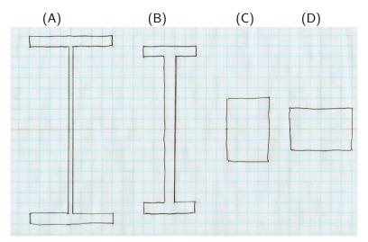
Each shape has the same area: 24 squares. Which shape has the **smallest**  $I_x = \int y^2 \mathrm{d}A$  ("second moment of area about the x-axis"), with y=0 given by the faint horizontal red line at the center?
