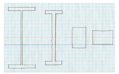
If you moved the x-axis down by a couple of grid units, what would happen to  $I_x = \int y^2 dA$  for each shape? Would  $I_x$  change? Would  $I_x$  change by the same amount for each shape?
