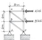
**2\*.** (Repeated/postponed from ws22/q4.) Using the method of sections, solve for the forces in bars *BC*, *CH*, and *FH* in the truss shown above (right). Your solution must include an EFBD for the half of the truss that you do not erase, with all external (or newly externalized) forces labeled. Indicate both the magnitudes of these forces and whether the bar is in tension or compression. [Warning: the angle of the 2 kN diagonal load is different from the angle of bar *CE*.]
