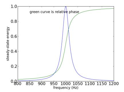
$f_0 = 1000$  Hz, Q = 100: energy and phase vs.  $f_{
