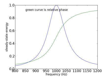
$f_0 = 1000$  Hz, Q = 30: energy and phase vs.  $f_{
