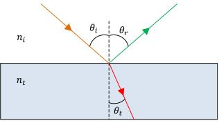
The angles that the incident (i) and reflected (r) rays make with the normal are the same. That is,  $\theta_i = \theta_r$ . The angles that the incident (i) and transmitted (t) rays make are related by Snell's Law:
