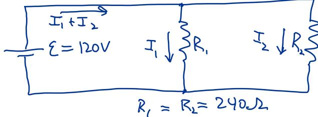
(e) How much current flows through each (individual) light bulb? (One way to work this out would be to use the junction rule and the loop rule, but you can use whatever method you prefer.)
