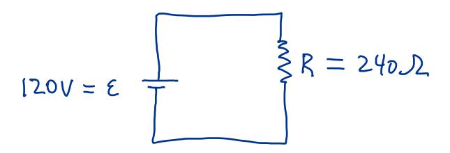
(b) What current flows through the  $240\,\Omega$  light bulb? (Use correct units!)
