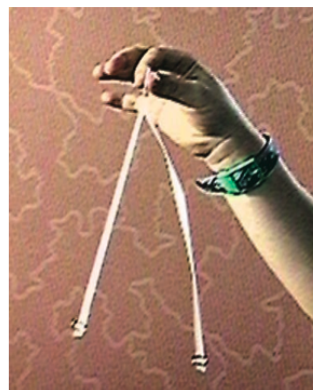
Figure 22.2 Strips of tape just pulled out of a dispenser repel each other. The repulsive force is large enough to keep the strips apart even when they are weighted down by paper clips.
