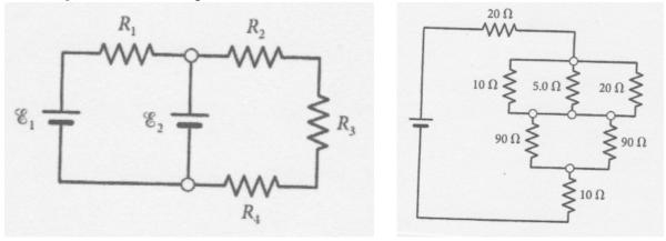
9. In the right figure above, the battery voltage is  $\mathcal{E} = 10$  V. (a) How much current flows through the battery? (b) How much power is supplied by the battery?
