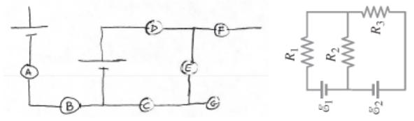
7<sup>\*</sup>. Determine the magnitude and direction of the current in each resistor shown in the right figure above. The batteries' emfs (i.e. their "voltages") are  $\mathcal{E}_1 = 9.0$  V and  $\mathcal{E}_2 = 12.0$  V. The resistors have values  $R_1 = 25 \Omega$ ,  $R_2 = 18 \Omega$ , and  $R_3 = 35 \Omega$ . Be careful with the orientations of the batteries. You should draw your own diagram of the circuit so that you can label the currents.
