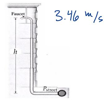
(b) Using Bernoulli's equation, calculate the **gauge pressure** in the pipe on the top floor. (This is within the pipe, before the faucet, so the water need not be at atmospheric pressure.)
