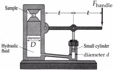
(a) Find the **force** exerted by the large cylinder on the sample. [Hint, in case you were not in Physics 8: the  $F_{\text{handle}} = 360 \text{ N}$  force at the end of the lever causes a  $2F_{\text{handle}} = 720 \text{ N}$  downward force to be applied to the small cylinder, as a result of the torque and the 2:1 lever-arm ratio.]
