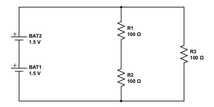
First, identify all of the **branches** in the circuit. For each branch, choose a **reference direction** for the current through that branch. How many branches? How many junctions?
