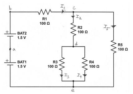
I count 4 loops. Let's see what the loop rule tells us. Again, one equation will be redundant. We'll just write down the equations, without wasting time to solve them for  $I_1 \dots I_5$ .
