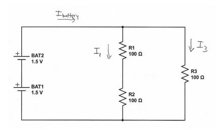
There are 3 loops in this circuit. Where are they? Use the loop rule for each one. (Let's go clockwise around each loop — arbitrary choice.) How many of these 3 equations give us new information?
