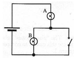
(A) an open switch has a very small resistance, effectively "zero"(B) an open switch has a very large resistance, effectively "infinite"
