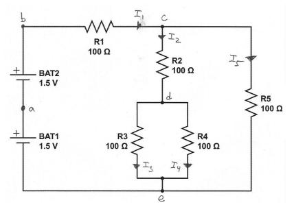
$l_1 = 0.01875 \text{ A}, \ l_2 = 0.0075 \text{ A}, \ l_3 = l_4 = 0.00375 \text{ A}, \ l_5 = 0.01125 \text{ A}$  $l_1R_1 = 1.875 \text{ V}, \ l_2R_2 = 0.75 \text{ V}, \ l_3R_3 = l_4R_4 = 0.375 \text{ V}, \ l_5R_5 = 1.125 \text{ V}$
