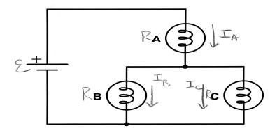
$$I_{A} = \frac{\mathcal{E}}{R_{A} + \left(\frac{R_{B}R_{C}}{R_{B} + R_{C}}\right)}$$
