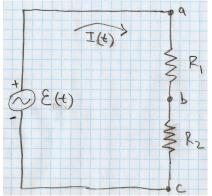
In series, each resistor (or light bulb) gets only a fraction of the total emf. So light fixtures are always in parallel, not in series (except holiday lights, etc.).  $\mathcal{E}(t) - I(t)R_1 - I(t)R_2 = 0$
