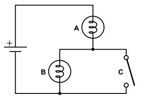
$$I_{A} = \frac{\mathcal{E}}{R_{A} + \left(\frac{R_{B}R_{C}}{R_{B} + R_{C}}\right)} \qquad \text{If } R_{A} = R_{B} = R \neq 0 \text{ and } R_{C} = \infty \text{ then}$$
