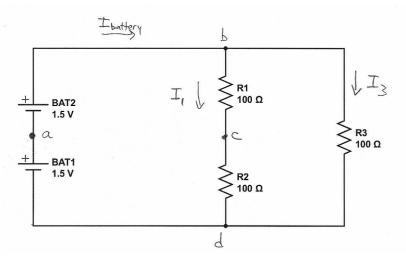
One more question: What is the power dissipated in each resistor? (Are they all the same, or not?) What is the power supplied by each battery?
