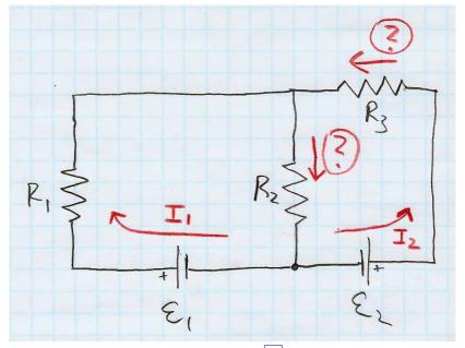
What values can we write for the two 2 currents? What does the loop rule tell us? (3 equations, but 1 is redundant.)
