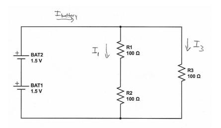
What does the **junction rule** let us write for the junction above  $R_1$ ? In this case, do we get any additional information by applying the junction rule at the junction below  $R_2$ ?
