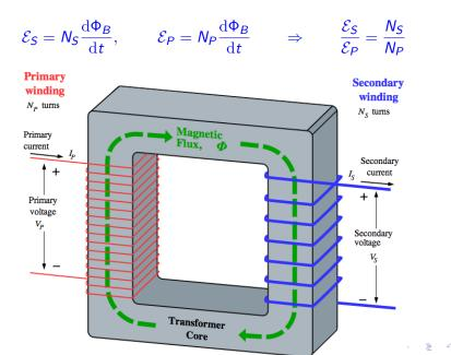
Consider an ideal step-down transformer in which the primary coil has 1000 turns and the secondary coil has 100 turns. The primary is connected to an AC power source, and the secondary is connected to a light bulb. If the rms voltage delivered by the AC power source is 120 volts, what is the rms voltage across the bulb?
