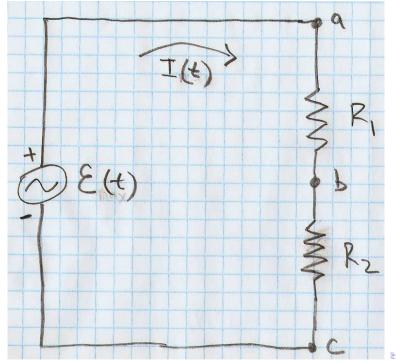
The usual "junction rule" and "loop rule" work for AC too, but voltage and current are functions of time now.
