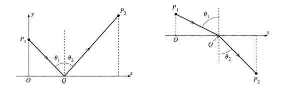
**XC4\*.** Optional/extra-credit. A ray of light travels from point  $P_1$  in a medium of refractive index  $n_1$  to  $P_2$  in a medium of index  $n_2$ , by way of the point Q on the plane interface between the two media, as in the right figure
