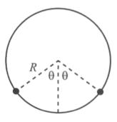
**XC3\*.** Optional/extra-credit. Two equal masses are glued to a massless hoop of radius R that is free to rotate about its center in a vertical plane. The angle between the masses is  $2\theta$ , as shown in the right figure above. Find the frequency of small oscillations. (This is an easy XC problem.)
