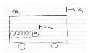
A cart of mass  $m_1$  rolls horizontally without friction. The cart's position is  $x_1$ . Inside the cart, a mass  $m_2$  is attached to the wall of the cart with a spring (constant k). The position of  $m_2$  w.r.t. the spring's relaxed position is  $x_2$ . So  $x_2$  is w.r.t. the cart, not w.r.t. the ground. Write  $\mathcal{L}(t,x_1,\dot{x}_1,x_2,\dot{x}_2)$ .
