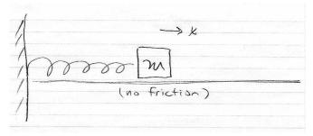
OK, how about a block of mass m moving horizontally on a frictionless table, under the influence of Hooke's-Law potential
