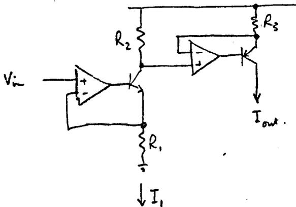
$$I_1 = \frac{V_{in}}{R_1} \quad \text{since } + \text{ and } - \text{ inputs are at same potential.}$$
