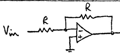
$$\frac{V_{in}}{R} = -\frac{V_{out}}{R} \Rightarrow V_{out} = -V_{in}$$
