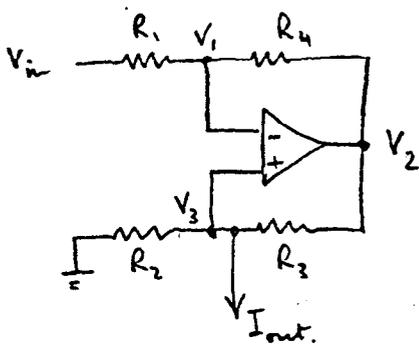
When op amp is balanced  $V_1 = V_3$
