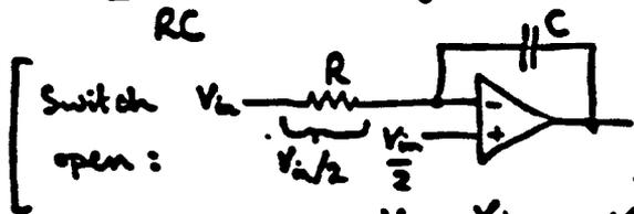
Rate (open) =  $\frac{V_{in} - \frac{V_{in}}{2}}{RC} = \frac{V_{in}/2}{RC}$
