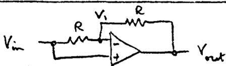
$$\left. \begin{array}{l} V_1 = V_{in} \text{ balance} \\ \frac{V_{in} - V_1}{R} = \frac{V_1 - V_{out}}{R} \end{array} \right\} \Rightarrow V_{out} = V_{in}$$
