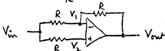
$$\left. \begin{array}{l} V_1 = V_2 \text{ balance} \\ V_{in} = V_2 \text{ assuming no bias current} \\ \frac{V_{in} - V_1}{R} = \frac{V_1 - V_{out}}{R} \end{array} \right\} \Rightarrow V_{out} = V_{in}$$
