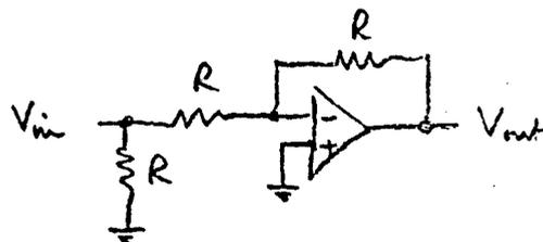
$$\text{As above: } V_{out} = -V_{in}$$
