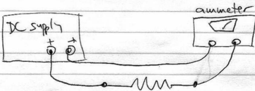
Setup for measuring  $I$  vs.  $V$
