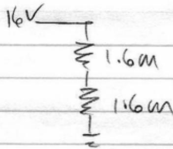
I inserted ammeter between lower resistor & ground. Measure  $\approx 5\mu A$ .
