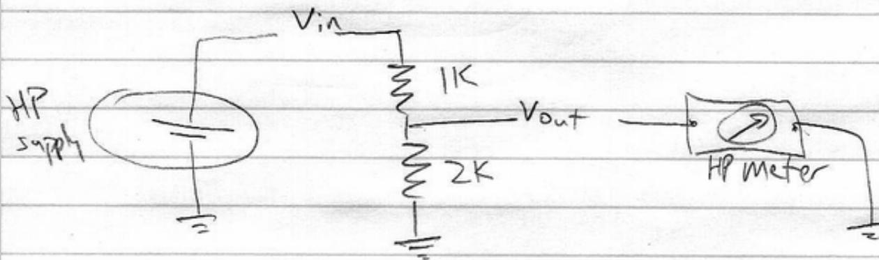
Set  $V_{in} = 3.0V$  from  $+25V$  supply
