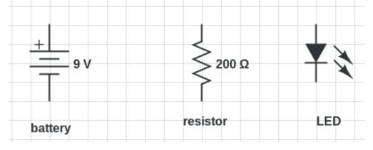
In the space below, draw a schematic diagram for a circuit in which the battery, the 200  $\Omega$  resistor, and the red LED are all connected **in series**. Try to orient the battery and LED symbols such that the LED will light up. Check with your neighbors to see if you all have similar diagrams! (Draw your schematic diagram in the space below.)
