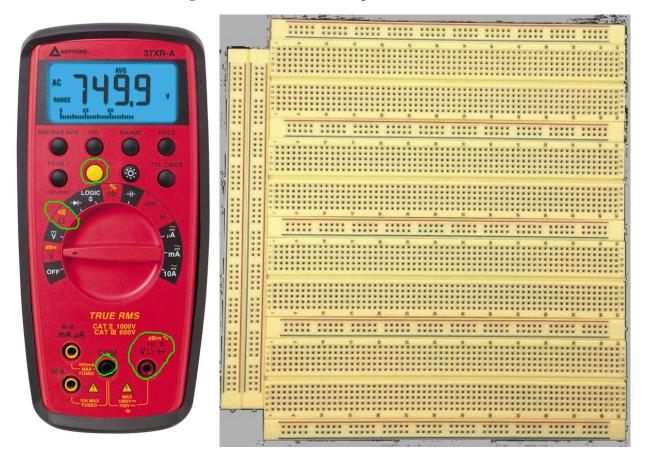
Use the Amprobe hand-held meter (shown above-left) to figure out which holes in the breadboard (shown above-right) are internally electrically connected to one another. The easiest way to connect the meter to the breadboard is to use cables that have a "banana" connector on one end (left photo below) and a spring clip (right photo below) on the other end.
