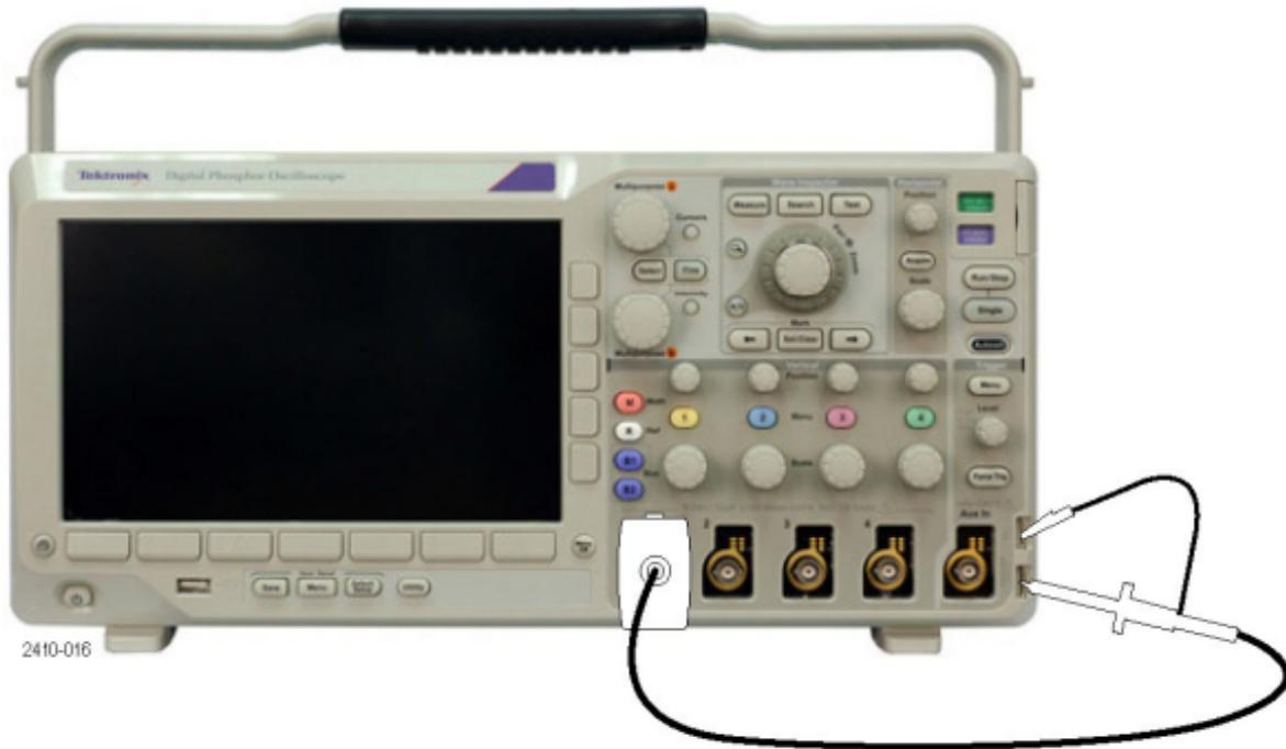
1.1 Connect the probe as shown in the photo above. The lower-right clip on the scope outputs a 1 kHz square wave, while the upper-right clip is grounded. Adjust the probe with a small screwdriver until the square wave looks square. First try turning the screw in one direction to exaggerate the high frequencies, then in the other direction to attenuate the high frequencies, and then finally to get the square wave just right.
