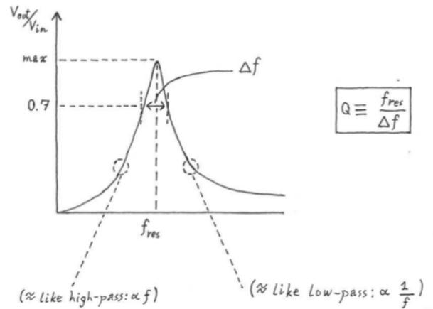
On page 7 of last week's notes ("reading02.tex" due 9/7), we saw the *band-pass* filter shown above (left). It again looks like a generalized voltage divider, where the impedance on top is  $\mathbf{Z}_1 = R$  and the impedance on the bottom is
