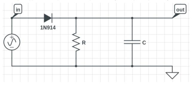
Use the above half-wave rectifier, with capacitor included, to extract the envelope from the FG's amplitude-modulated waveform. Use  $R = 10 \text{ k}\Omega$  and  $C = 1 \mu\text{F}$ , to get RC = 10 ms, which is several times the 2.3 ms period of the 440 Hz tone that the FG is modulating.
