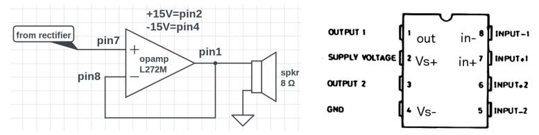
Look with the oscilloscope at the follower input and output, both before and after connecting the speaker. If all goes well, the signal reaching the speaker should be a pleasant 440 Hz sine. If not, ask us for help!
