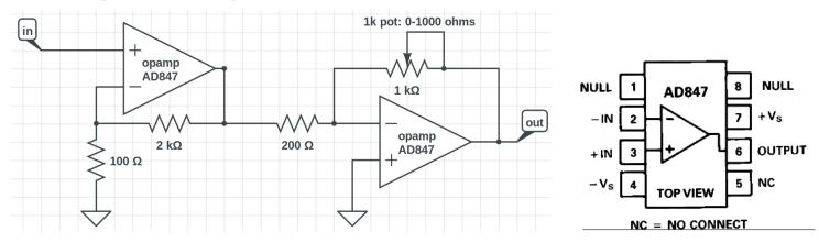
After double-checking that the output of your LC filter is less than about 1 V<sub>pp</sub>, connect the output of the filter to the input of the amplifier, and see if the opamp's  $V_{out}(t)$  is a faithfully amplified copy of your amplitude-modulated signal. If not, ask for help. Check that you're able to adjust the amplitude of  $V_{out}$  by dialing the gain via the potentiometer.
