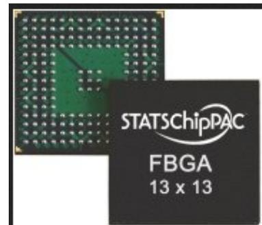
By the way, if you actually look through the `basys2.ucf` file in your web browser or in the Xilinx ISE software, you'll see that its main purpose is to assign human-readable names (like `led`, `sw`, `btn`, `seg`) to the FPGA's built-in input/output pins. The bottom of the FPGA looks something vaguely like the above-right picture. (This is not exactly the same pattern as the FPGA on your board, but it illustrates the same idea.)
