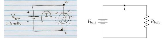
If you imagine the wires to be thick copper at room temperature and the bulb's filament to be extremely thin tungsten at  $T \approx 3000$  K (for most materials,  $\rho$  increases with T), the resistance of the copper wires is negligible in comparison to that of the filament. We usually draw "schematic" circuit diagrams in which idealized wires have zero resistance and pertinent electrical properties like resistance (and next week
