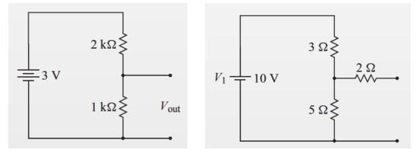
2. Find the Thevenin voltage  $(V_{\rm th})$  and Thevenin resistance  $(R_{\rm th})$  of the circuit shown in the right figure above. Explain to me how the  $R_{\rm th}$  calculation is done using each of the two methods explained in the text.
