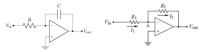
2. (a) If I choose  $R_1 = 2 \ k\Omega$  and  $R_f = 20 \ k\Omega$  in the above-right circuit, what is the relationship between  $V_{\text{out}}$  and  $V_{\text{in}}$ ? (Try to get both the magnitude and the sign right.) (b) Assuming that the "golden rules" correctly describe this circuit's operation, what potential difference (voltage) is measured between point A and ground? (c) Again using the golden rules, what relationship can you write between  $I_1$  and  $I_f$ ?
